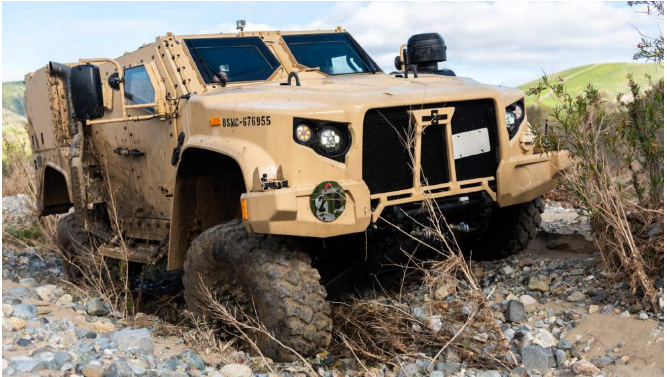
A Joint Light Tactical Vehicle displays its ability to handle multiple terrain types by physically adjusting its suspension during a demonstration at the School of Infantry West, Marine Corps Base Camp Pendleton, California, Feb. 27, 2019.
