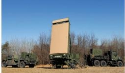
The G/ATOR is a three-dimensional, expeditionary, short/medium-range multirole radar capable of detecting low-observable, low-radar-cross-section targets such as rockets, artillery, mortars, cruise missiles, and manned
